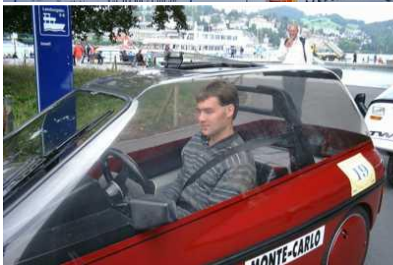
Ruedi Streuli from Switzerland presented his CityEl, which he converted with a new drive train, incorporating a range extender fuelled by methanol.
